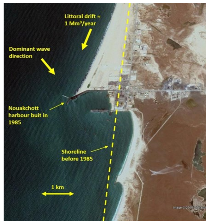
The seaport of Nouakchott (Mauritania) built in 1985 (Photo credit: Google Earth image & Job Dronkers). The port blocks the strong N-S littoral drift along the Mauritanian coast due to its orientation perpendicular to the dominant wave direction. The result is massive accretion at the updrift side and equivalent massive erosion at the downdrift side of the harbour.
