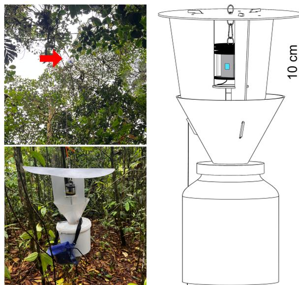
Fig. 2: Photographs of the funnel trap set up in the canopy (red arrow) and understory, and 3D model of a trap. Egg cartons and chloroform supply are placed inside the bucket. The blue bag stores the battery. On top of the trap is a roof extension (not shown in the 3D model).
