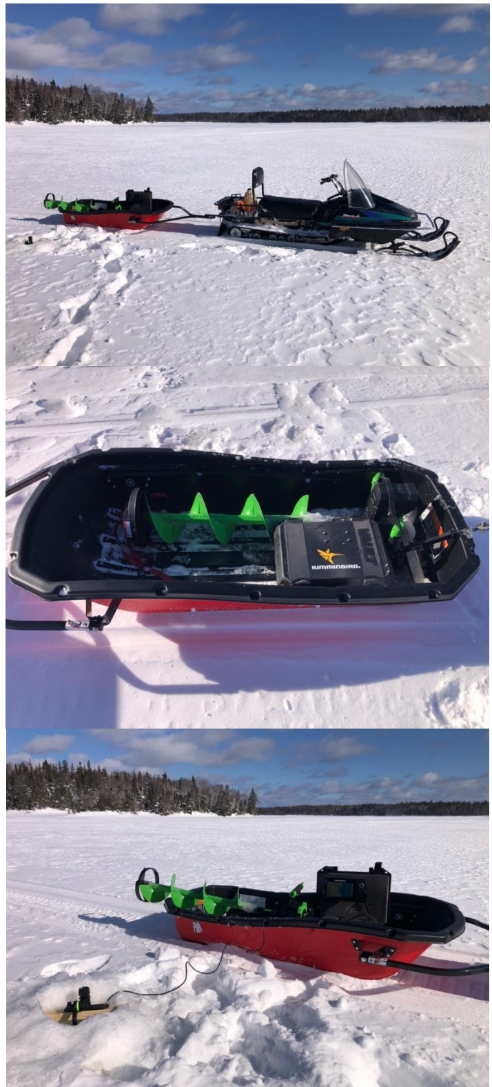
Figure 25. Setup for surveying depths of lakes. Depending on lake surface area, up to 150 holes were drilled with a large electric auger in a grid pattern. A transducer mount was lowered through the hole and point source sonar data was taken. When relatively deep water was found, more holes were drilled to determine maximum depth in the area. Depths were calculated from Humminbird® Autochart Pro software. Images February 20/24.
