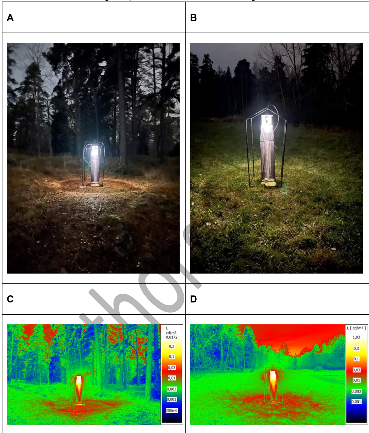
3 Figure B1. a) Photo of the insect light trap in forest. B). Photo of the insect light trap in the open meadow. c) 4 Luminance photo of the insect light trap in forest, d) luminance photo of the insect light trap in the open meadow.
