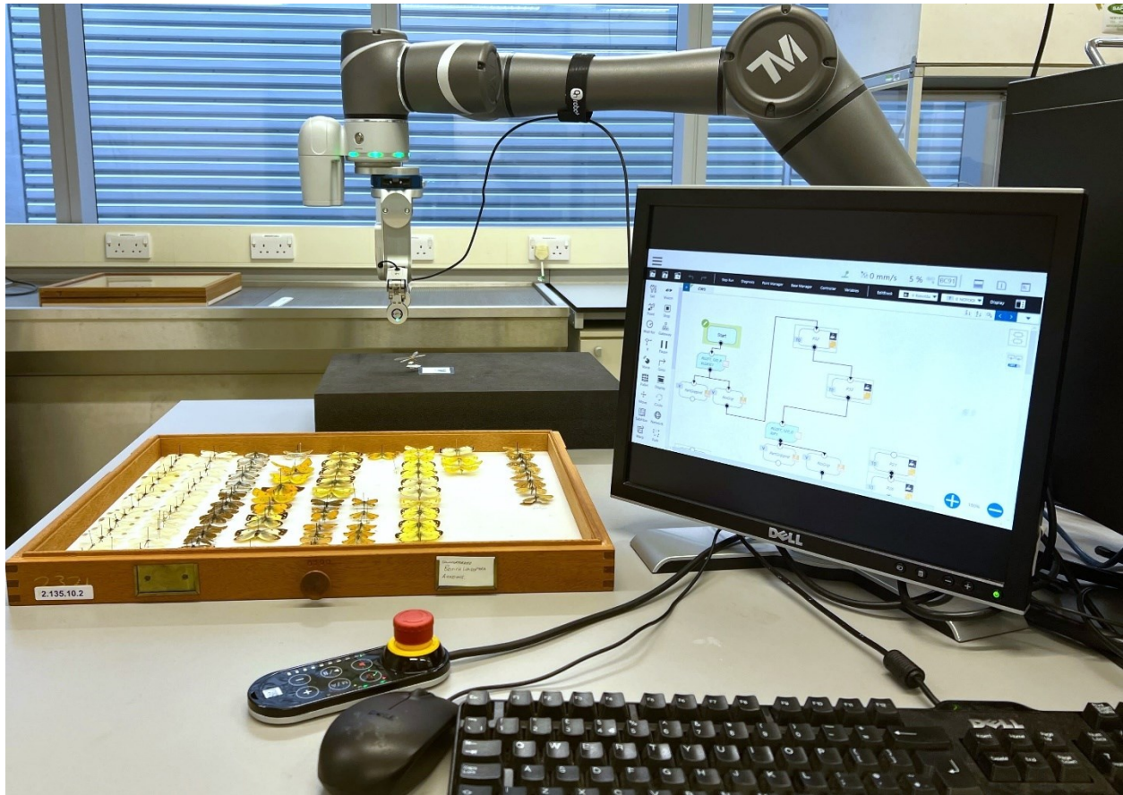
Figure 6. A Techman 500 robotic arm in action at the Natural History Museum, London, placing down a sample pinned specimen from a Lepidoptera collection. Here, the robotic arm has been trained to locate the specimen from the drawer, and then pick it up and place it on a board in order to scan the specimen. Synthetic specimens were used in the training stage for this task.
