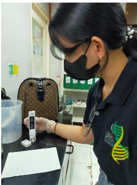
Figure E2. Total dissolved solids and electrical conductivity measurement.
