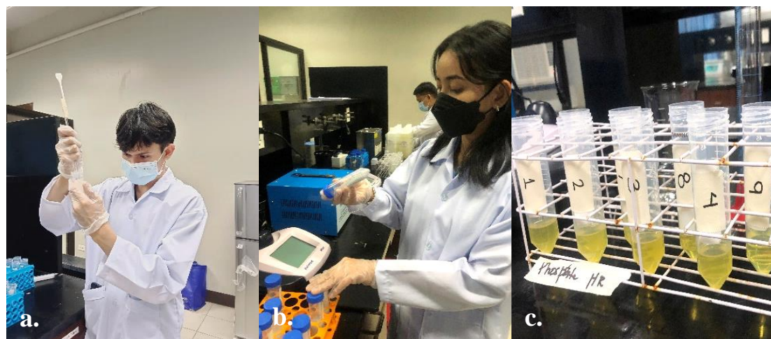
Figure E6. Phosphate measurement. (a) addition and crushing of reagents; (b) inversion and mixing of tubes; (c) color development.
