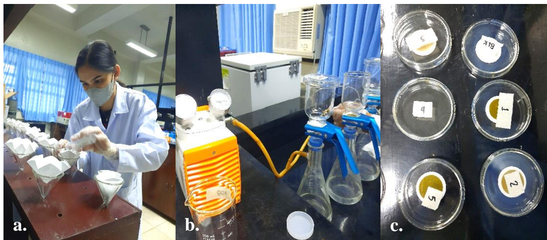
Figure E3. Total suspended solids measurement: a) straining reagent residues; b) filtration apparatus; c) Whatman™ membrane filters after filtration.
