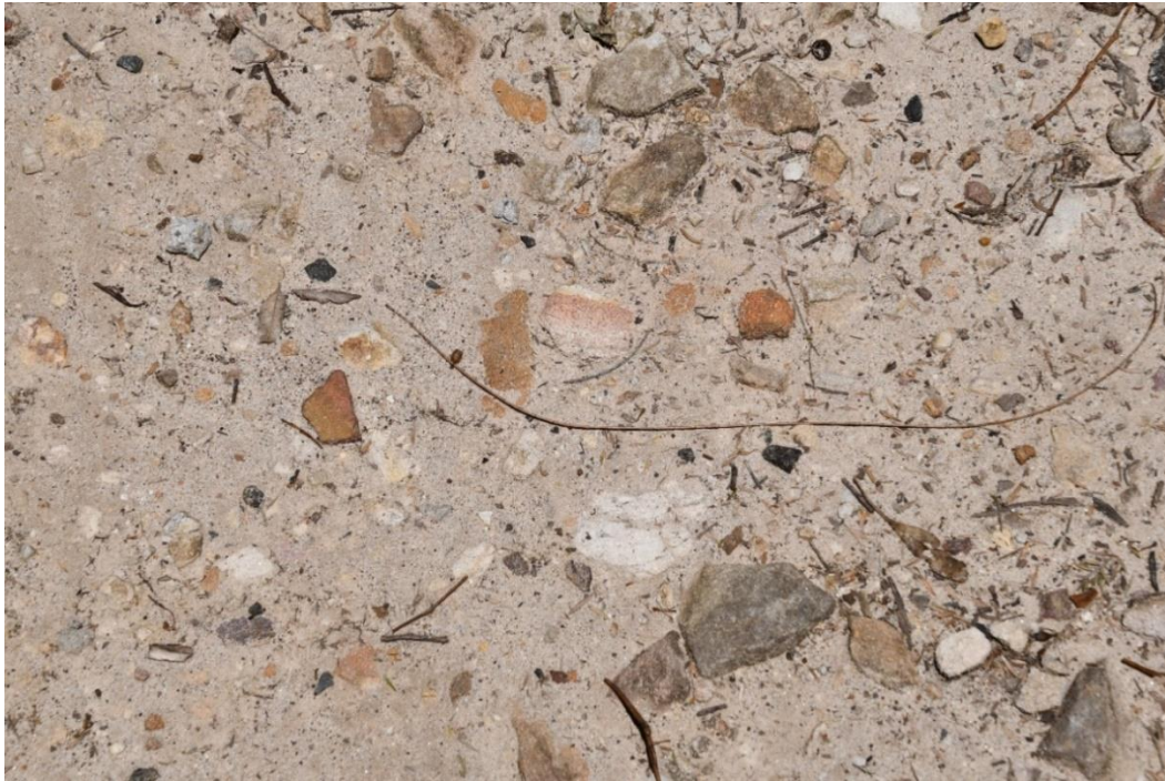
Close-up of the exposed soil just north of the central bridge, showing evidence of the Minchinbury Sandstone deposit.
