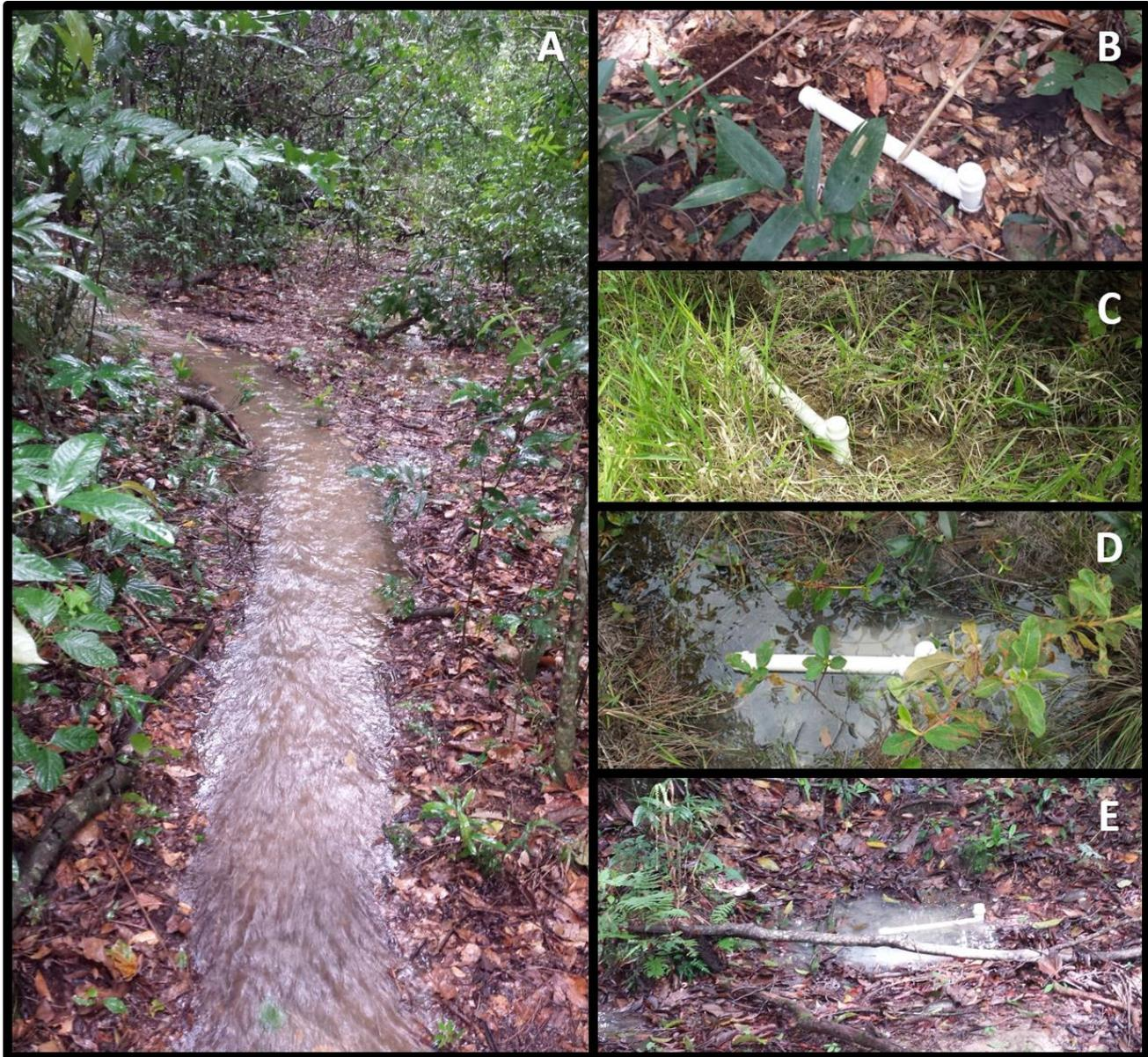
**Figure S1.** A) one example of surface runoff pathway from the cropland into the riparian zone; B and C) overland flow detectors in the gallery forest and *campo de murundus*, respectively, and; D and E) overland flow detectors few minutes after a rainstorm in the border between the cropland and the riparian zone and in the gallery forest, respectively.
