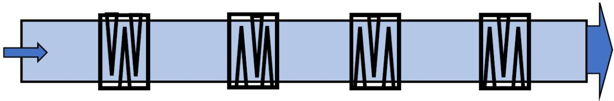
**Figure S1.** Artificial indoor flow-thru channels (length 6 m, width 0.4 m, depth 0.2 m, flowrate 1.60 L s<sup>-1</sup>) with added gravel (appr. grain size 50mm) in the bottom. In both ends there were a metal grid (mesh  $\text{\O} = 5$  mm). Each channel was equipped with four PIT-antenna coils (black lined areas) covering half a metre area each. The thin blue arrow indicates the water inlet and the thick blue arrow indicates the water outlet.
