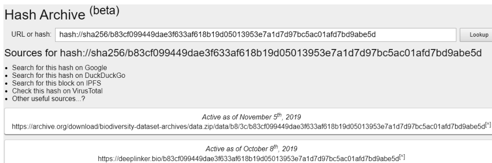
Figure 5. An example of a search index mapping hashes to archives. A search for a content or provenance hash at hash-archive.org will find any associated URLs that have been registered at hash-archive.org.
