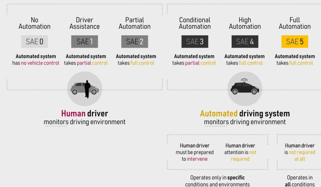
Figure 1. The six levels of AV automation defined by the Society of Automotive Engineers (SAE), ranging from 0 (fully manual) to 5 (fully autonomous).
