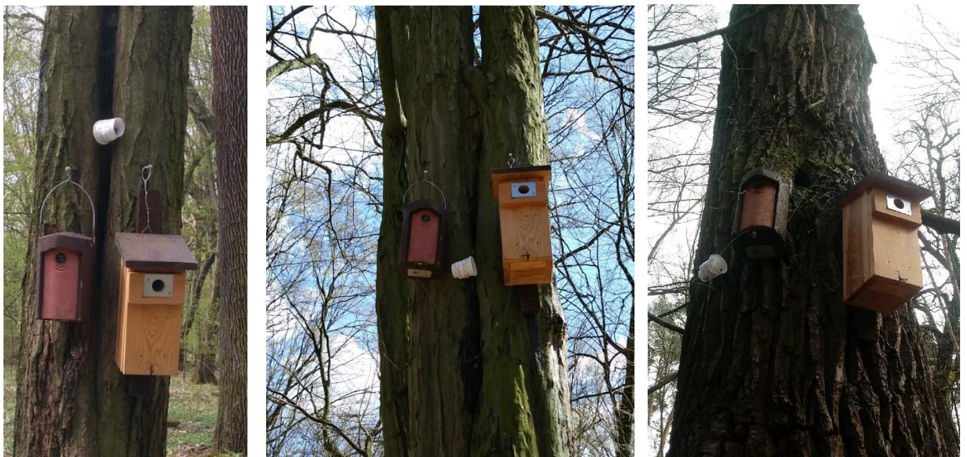
Figure S1. Examples of experimental setup to measure temperature and humidity at nest-site choice (early spring) in the different types of nests. Loggers, used to measure ambient conditions, were covered with a thick white plastic cup, open on both ends, to avoid direct sunlight and precipitation.
