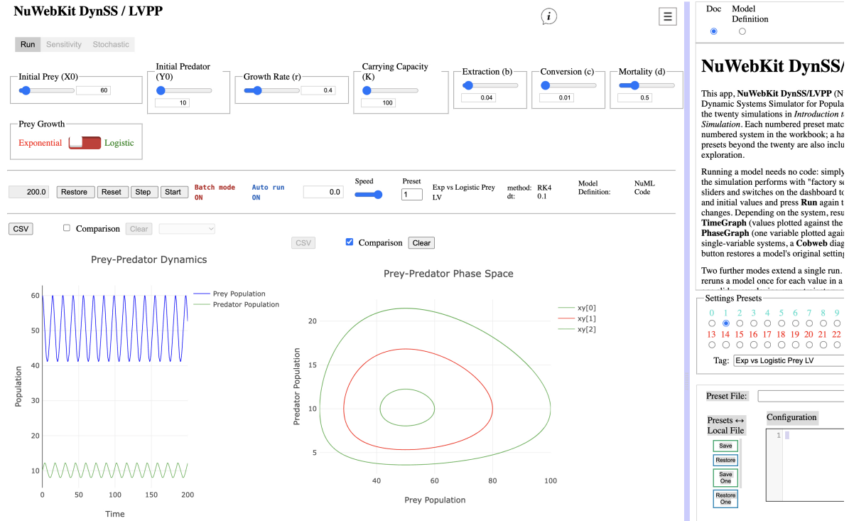
Figure 1. The NWK DynSS LVPP dashboard (to the left of the vertical light purple line) running the Lotka-Volterra prey-predator preset (Preset 1). Sliders set parameter values and initial conditions; the run ribbon shows the integration method and step size; and the time and phase-plane graphs update as the simulation runs. The sliders show the factory settings of the preset, except that initial prey density is set to 60 for the last of the three runs, and the right-hand graph shows the prey-predator phase space for three runs of the classical model with exponential prey growth (Module 1), started from (x_0, y_0) = (100, 10) (outer green; factory setting), (80, 10) (red) and (60, 10) (inner green). The drawer icon ( \equiv , upper right of the dashboard) opens the windows to the right of the purple line, here partly cut off: documentation above, and the bank of presets (0-9 factory, 10-25 user) with buttons for saving presets to, and restoring them from, a local file below. Selecting the Model Definition radio button at the top of the drawer opens two further windows, one describing the model and the other holding its NuML code (Fig. 2).
