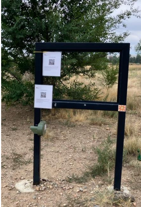
Figure 2: Trail counter affixed to the left metal post at the Northeast trailhead at South Loop Drive’s parking lot, along with the survey solicitation and QR code.
