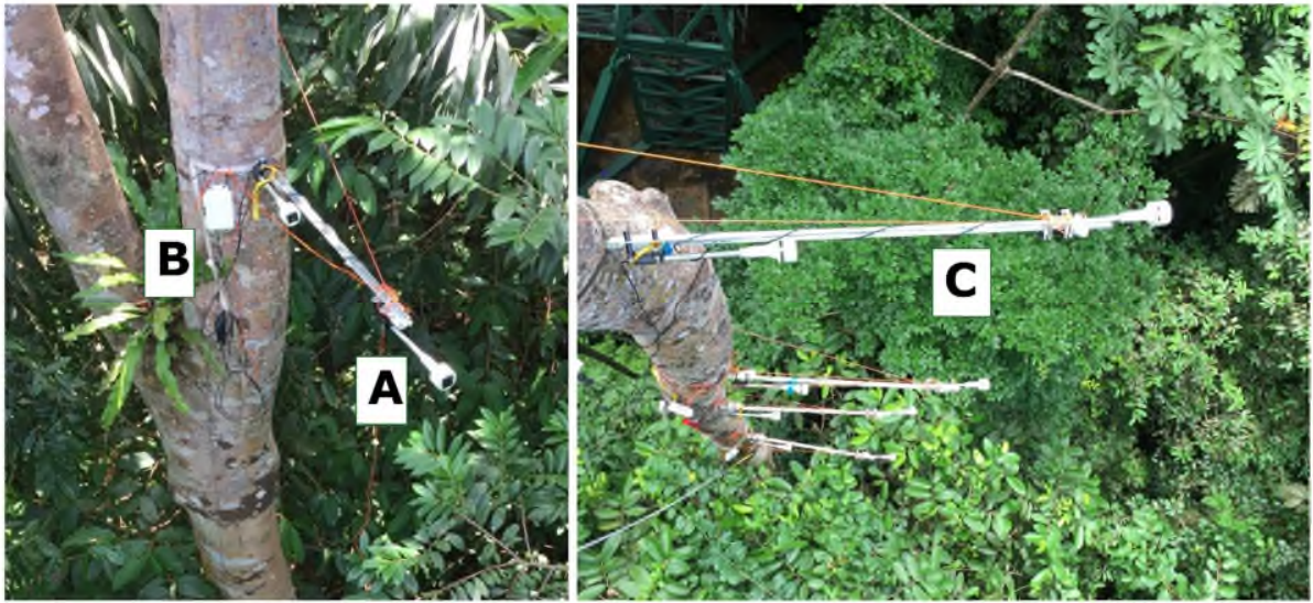
Figure S4. Assessing wind dynamics along the forest height gradient. Sonic anemometers ( A ), screwed to an aluminium frame at two positions (in = near the stem, out = 1.35 m away from the stem), were strapped to stems or branches of trees at four heights to measure winds, gusts, and wind direction for 3- to 10-second intervals (0.3 to 0.1 Hz) for one to five consecutive days. Loggers ( B ) logged the measurements. Every anemometer was additionally coupled with a temperature sensor ( C ). The images were taken by MH.
