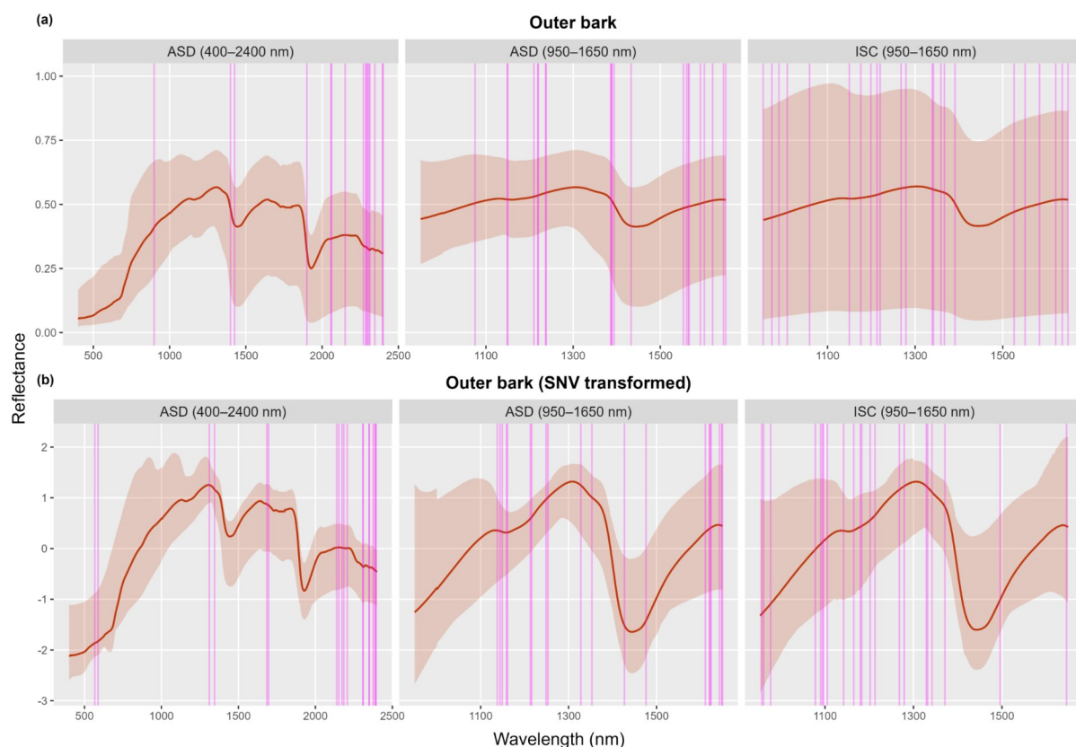
Fig. S11. Raw (a) and preprocessed (b) spectral reflectance of outer bark of standing trees measured with ASD FieldSpec® 4 and ISC NIR-S-G1. Dark brown (a) and orange (b) lines represent the mean reflectance, while shaded areas indicate the full range (minimum to maximum) of reflectance values. Vertical pink bands highlight wavelengths identified as most informative by LDA-based variable selection.
