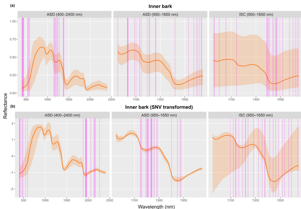
Fig. S12. Raw (a) and preprocessed (b) spectral reflectance of inner bark of standing trees measured with ASD FieldSpec® 4 and ISC NIR-S-G1. Dark brown (a) and orange (b) lines represent the mean reflectance, while shaded areas indicate the full range (minimum to maximum) of reflectance values. Vertical pink bands highlight wavelengths identified as most informative by LDA-based variable selection.
