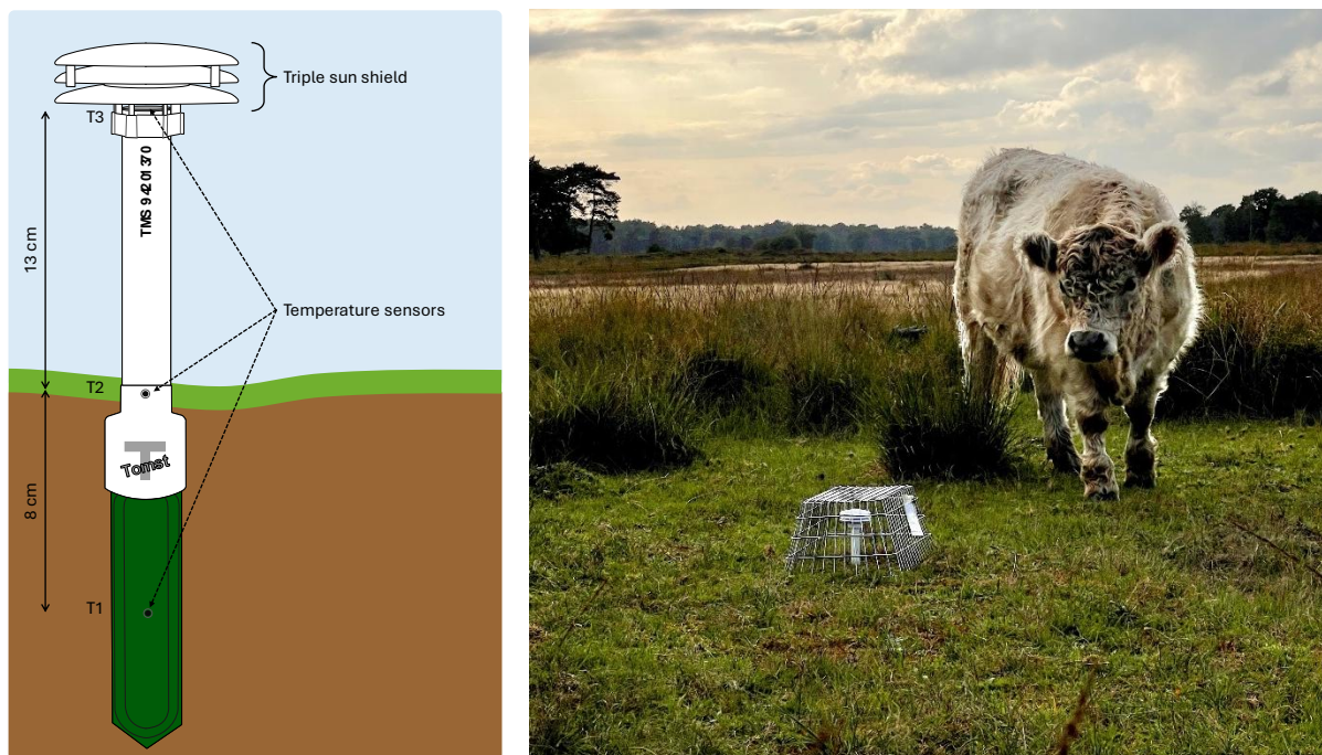
1064 Figure A1. Schematic view (left) and picture in the field (right) of a TOMST TMS-4 logger. The TOMST TMS-4 loggers were 1065 placed in the field, covered by a chromed steel shopping basket to protect them against grazers. The sensors were placed with 1066 the middle temperature sensor (T2) facing north and making contact with the ground. Left image inspired by Wild et al. 1067 (2019).
