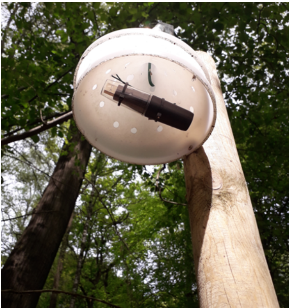
Figure 4: Lascar logger with a self-made double radiation shield, made from two white funnels. The inner funnel has holes to stimulate air flow. Pictures from Pieter De Frenne
