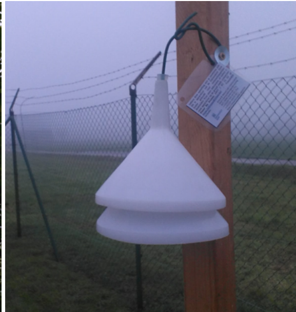
Figure 4: Lascar logger with a self-made double radiation shield, made from two white funnels. The inner funnel has holes to stimulate air flow. Pictures from Pieter De Frenne
