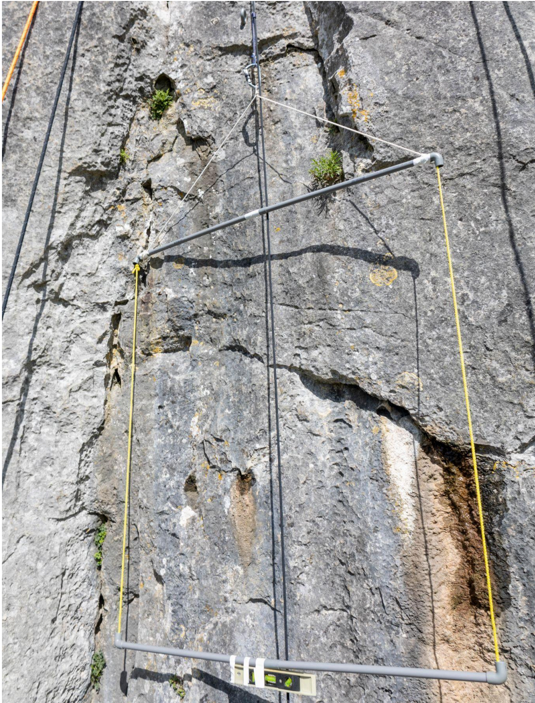
Figure 5: Fixed frame connected with a prusik knot to a second rope
