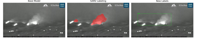
Fig. 6: Nighttime scenario: while the base model did not identify smoke, SAM2 successfully segmented the plume and propagated the labels through low-light conditions.
