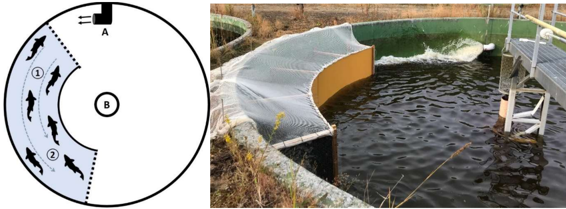
Figure S1: Top view of the tanks. Coloured area represents the cage that constrained the fish to swim at the desired speed. Number 1 & 2 represent the two points where the speed of water were measured at the surface and at the bottom. Letter A correspond to the water inflow. Letter B represent the central column with the outflow. B) representative picture of a fish tank.
