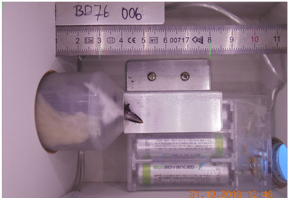
Figure 3: The green lines are selected by user, 5 cm apart and used to find the pixels to mm conversion factor
