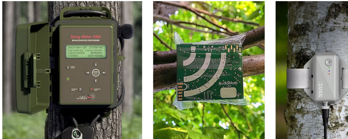
Figure 3. A commercial ARU, the SM4 from Wildlife Acoustics (left), and two open-source units, the AudioMoth (centre; pictured here in low-cost waterproofing) and the Bugg (right).
