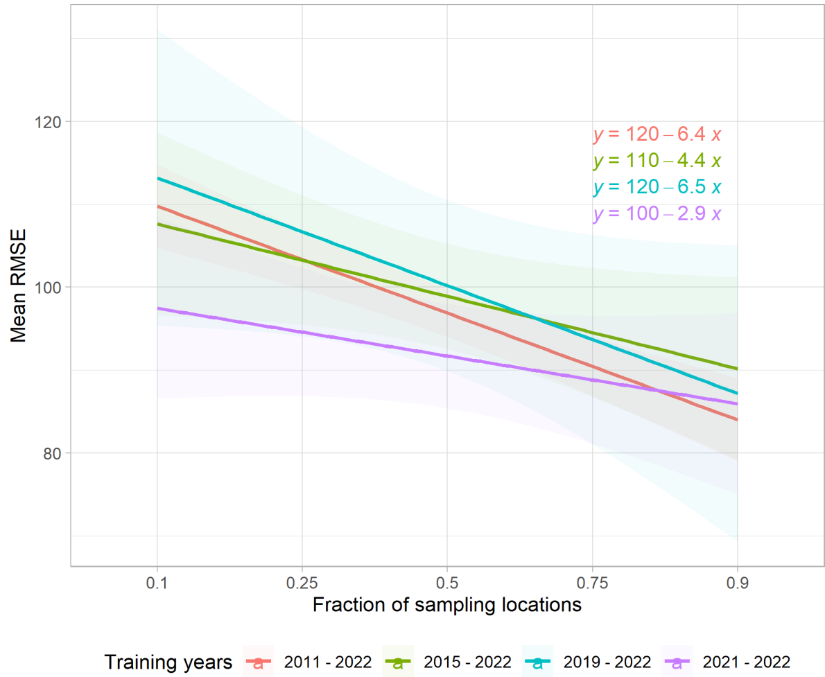
Figure 3: Linear model plot showing the relationship between the fraction of sampling locations and the mean RMSE for different training year sets (2011-2022, 2015-2022, 2019-2022, and 2021-2022). C.I. is 95%. The trend is similar across the four training year groups: as the fraction of sampling locations increases, the mean RMSE consistently decreases across all training year sets, indicating that higher fractions of sampling locations improve model accuracy.
